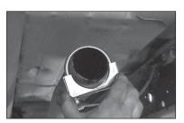
11. Install the 2-1/2" clamp (E) over stock pipe.
