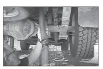
6. Remove tailpipe assembly from rear of vehicle.
