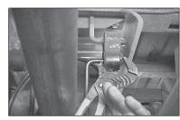
9. With muffler properly supported, using a pair of channel lock pliers, remove front muffler hanger rods from lower hole in rubber grommets.
