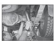
15. Install tail pipe (C) from rear of vehicle with short end of tube towards rear of muffler (B).
