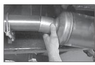
14. Install muffler (B) over head pipe (A) with JBA logo facing rear of vehicle making sure slip joint is bottomed out.
