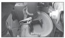
3. With vehicle raised and properly supported, using a reciprocating saw or hack saw, cut tail pipe off at rear of muffler in front of hanger rod.
