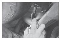
4. Spray lubricant on front and rear tail pipe hanger rubber grommets.
