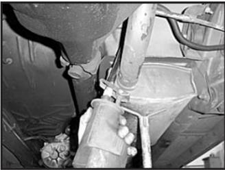
3. With the vehicle raised and properly supported, use the reciprocating saw to cut the weld at the rear of the muffler. Remove the factory tailpipe.
