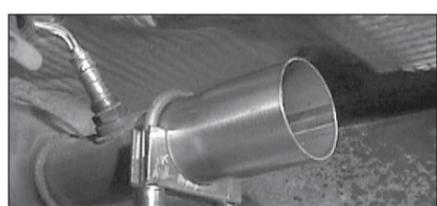
10. Install 2 1/4" clamp (D) over head pipe (A) slip joint, and tighten completely using a 9/16" socket. NOTE: USE ANTI SEIZE ON THREADS. SEE NOTE: #2
