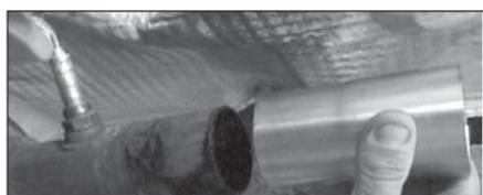
9. Reinstall oxygen sensor. Install JBA head pipe (A) aligning notch with locating pin. NOTE: You may have to tap on with rubber mallet.
