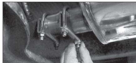
12. Install and position 2-1/2" clamp (E) over muffler front slip joint, and hand tighten only at this time. NOTE: USE ANTI SEIZE ON THREADS. SEE NOTE: #2
