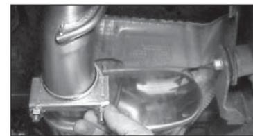
17. Install and position 2-1/2" clamp (F) over rear muffler slip joint, and hand tighten only at this time. NOTE: USE ANTI SEIZE ON THREADS. SEE NOTE: #2
