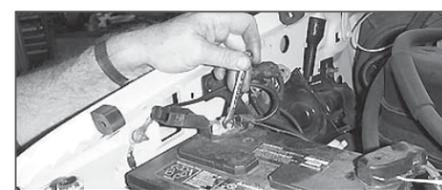
21. Lower vehicle and reattach the negative battery cable.
