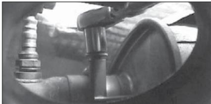
3. With vehicle raised and properly supported, remove clamp at front of muffler, using a 15mm socket.
