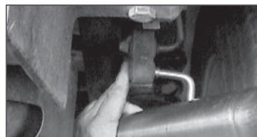
15. Install rear tail pipe hanger into lower hole of rubber grommet.
