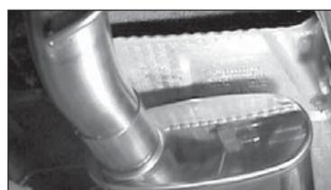
14. Install tail pipe into rear muffler slip joint.
