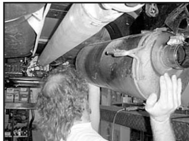
10. Remove factory muffler assembly.
