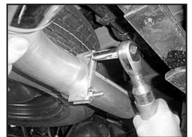
21. Align exhaust tip (D) properly and tighten clamp (F).
