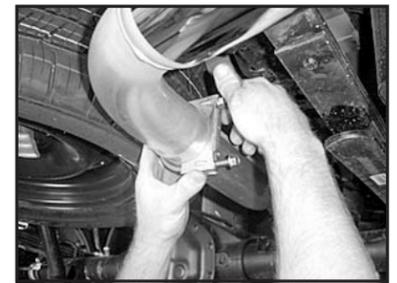
20. Position exhaust clamp (F) over exhaust tip (D).
