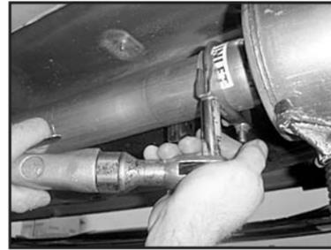
13. Insert muffler (B) into intermediate pipe (A). Place exhaust clamp with hanger (G) at the front of the muffler.
