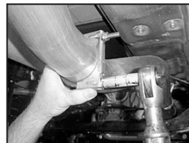
12. Install intermediate pipe (A) and secure with exhaust clamp (F).
