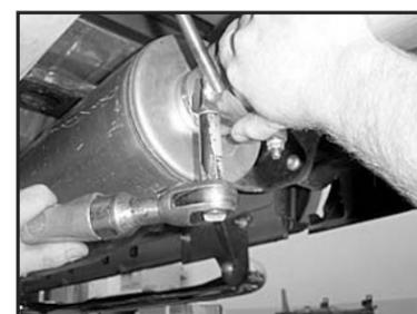
17. Align tail pipe (C) properly and tighten muffler hanger clamp (E).
