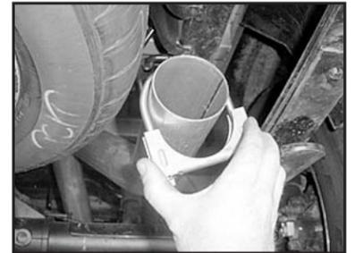
18. Install exhaust clamp (F) loosely over tail pipe (C). Do not tighten at this point.
