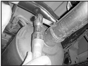
3. With the vehicle raised and properly supported, using the 15mm socket and ratchet, loosen the clamp, at the rear of the muffler, that secures the tail pipe to the muffler.
