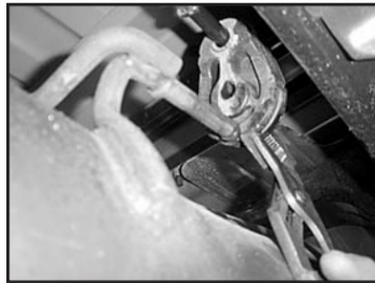
9. Remove muffer hangers from rubber isolators.
