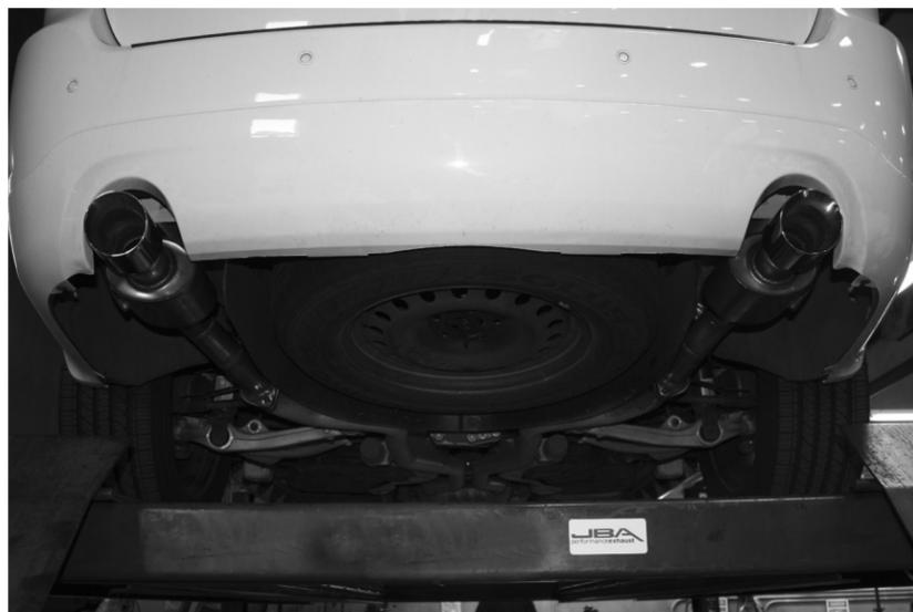
6. Remove the hangers from the rubber mounts and remove the muffler from the vehicle.
