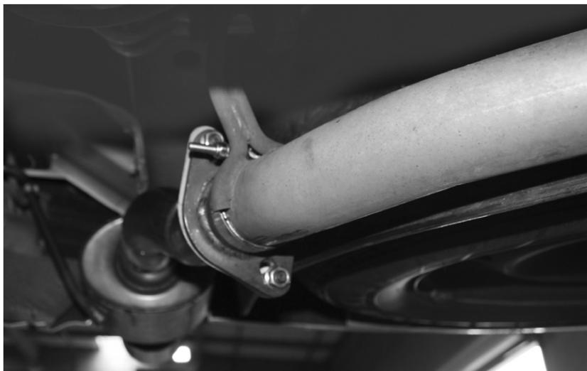
11. Align the Tip in the center of the opening and check that the tip length is the same as the drivers side. Slip the adaptor forward or back to get the tips even. When you are satisfied with the location, tighten the Clamp to 20 ft. lbs.
