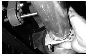
11. Slip the tail pipe with hanger (B) over the axle and insert it into the rear of the muffler (C). Insert the welded hanger on the tail pipe (B) into the rubber grommet.
