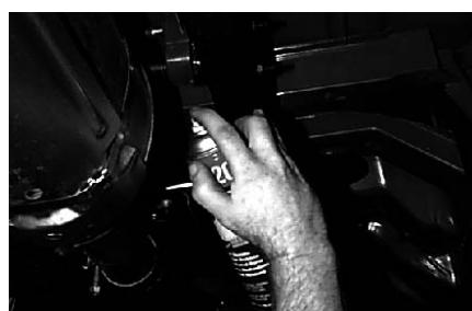
5. Spray lubricant on the hanger grommet at the front of the muffler, the one above the muffler and at the rear by the exhaust turn out.
