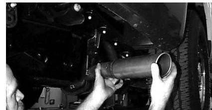
15. Check for adequate clearance from paint and body. With the turn out properly aligned, secure it in place with the 3" clamp (F) and tighten.
