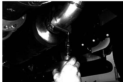
14. Install the turn out with tip (A) over the end of the tail pipe (B). Adjust the turn out so that it is level or slightly angled down.
