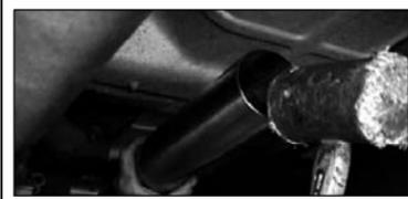
7. Slip 2-1/2" clamp (D) over end of head pipe (A). Install head pipe aligning notch with locating pin. Make sure pin is bottomed out in notch.
