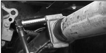
3. With vehicle raised and properly supported, remove front exhaust clamp using a 15mm socket.
