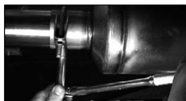
13. Position 3" clamp (E) over slip joint on front of muffler (B) and tighten completely using a 9/16" deep socket. NOTE: use anti seize on threads.
