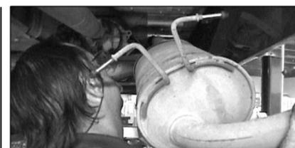
6. Using some form of heat and force, disengage and remove muffler assembly without damaging converter pipe.
