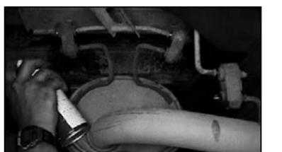
4. Spray lubricant on hanger rods in lower holes of rubber grommets at the tail pipe and end of muffler.
