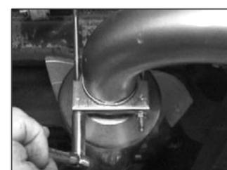
16. Using a 9/16" deep socket, snug nuts up on 3" clamp/hanger (F). NOTE: use anti seize on all threads.
