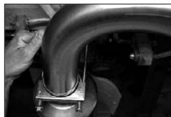
15. Slip tail pipe (C) into rear muffler slip joint, making sure it bottoms out.
