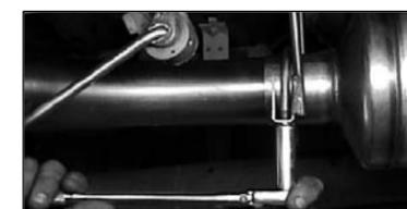
18. Tighten 3" clamp/hanger (F) completely using a 9/16" deep socket.
