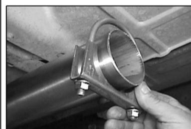
9. Install 3" clamp (E) over end of head pipe.
