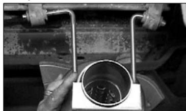
11. Position 3" clamp/hanger (F) over end of muffler (B) and hand tighten at this time.
