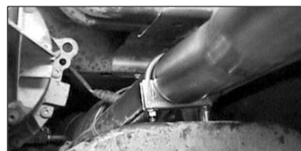
12. Position 2-1/2" clamp (D) over front slip joint on head pipe (A) and tighten completely using a 9/16" deep socket. NOTE: use anti seize on threads.
