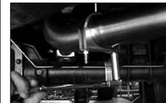
19. Install 3" clamp (H) over turn out slip joint and position 1/4" from lip. Tighten completely using 9/16" deep socket. NOTE: Use anti-seize on all threads of clamp. See note #2
