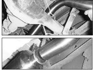
18. Install tail pipe (C) from rear of vehicle, and slip into muffler. Note: make sure that the end of the tail pipe with the hanger is at the rear of the vehicle.
