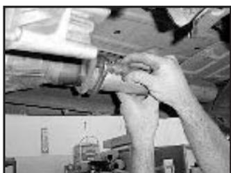
10. Using the factory fasteners and the supplied 2.25" clamp (G), install new intermediate pipe (A).
