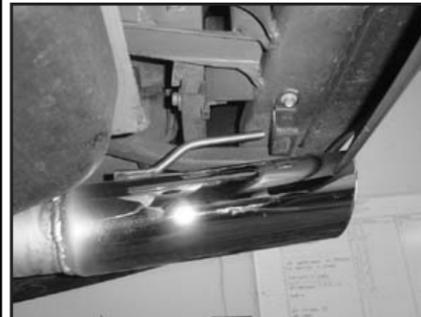
12. Install the JBA tail pipes (F) and (G) by first inserting the tip hanger into the rear rubber isolator.
