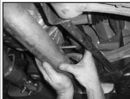
9. Slip the mid pipe hangers in to the factory rubber isolators.
