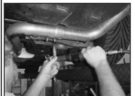
16. Secure band clamps (H) over slip connection.
