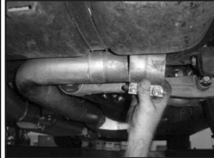
11. Slip 3" band clamp (H) over the end of mid pipes (D) and (E).
