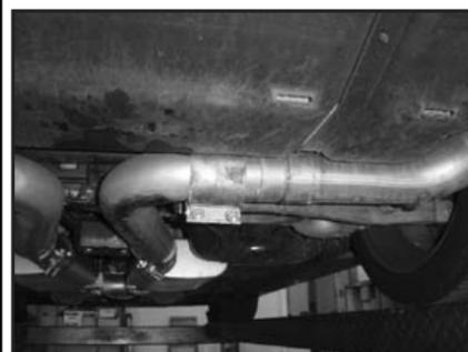
13. Now fully seat the tail pipes (F) and (G) on to the mid pipes (D) and (E).
