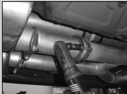
7. Align the mufflers and then tighten the fasteners that attach the intermediate pipes (A) and (B) to the catalytic converter assembly.
