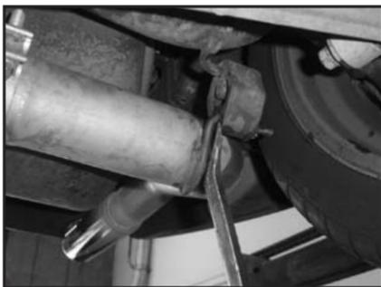
4. Using the pry bar, remove the tailpipe hangers from the rubber isolators.
