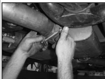
10. Install 3" exhaust clamp (I) over slip connection with muffler (C).
