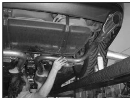
5. Remove the factory exhaust system by unbolting the intermediate pipes from the catalytic converter assembly.
