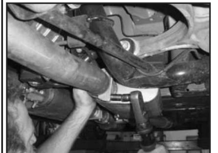
16. Check the exhaust system for proper alignment and clearance then tighten all clamps.
