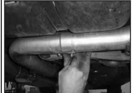
15. Position the band clamps (H) over slip connection.
