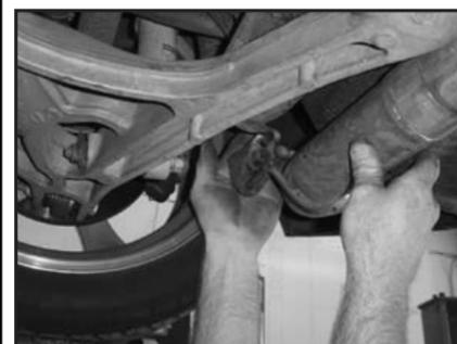
14. Slip 2nd tail pipe hanger into rubber isolator.
