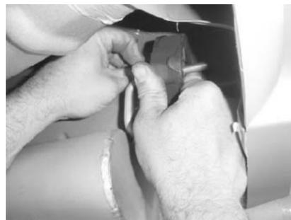
8. Install the new over axle pipes (B) and (C), slip a 2-1/2" clamp (H) onto each pipe, then insert into muffler/tip assemblies (D) and (E). Slip two ring clamps onto the Y-pipe (A), and insert the Y-pipe into the over axle pipes (B) and (C).
