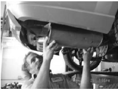
5. Using pliers or a pry bar, slide the rubber hanger from the hanger rod at inside, front of muffler (a little lube helps). Slide the muffler assembly forward and remove from slip hangers.
