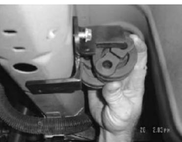
6. Bolt the supplied hanger brackets (G) to the frame on the drivers side using the supplied self tapping screws (I). Bolt the brackets in place with the factory holes. Prongs on the bracket need to face forward. Then slide two rubber isolators (F) onto each hanger so holes align.
