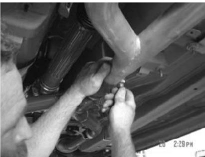
9. Using the factory clamp, attach the Y-pipe (A) to the converter assembly. Adjust to be flat to the ground, and tight to the converter assembly. Tighten securely.
