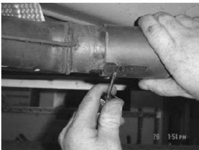
4. Loosen the clamp connecting the exhaust pipe to the muffler. Wiggle the exhaust pipe free from the muffler. Remove the exhaust pipe from car.
