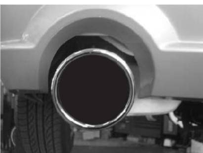
10. With the axle pipes (B) and (C) in the muffler assemblies (D) and (E) adjust mufflers to be flat, and the tips an equal distance from the bumper cover, Then tighten all clamps securely.
