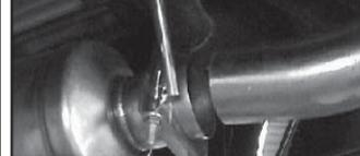
18. Install tail pipe (C) into rear slip joint on muffler (B). NOTE: tail pipe (C) should be installed with the hanger to the rear of the vehicle.
