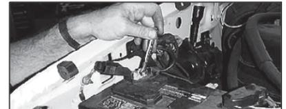
27. Lower vehicle and reattach the negative battery cable.
