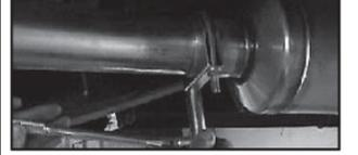
17. Position 3" clamp (E) on muffler (B) and using a 9/16" deep socket, tighten completely. NOTE: use anti-seize on threads.
