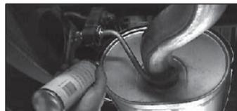
8. Spray lubricant on front muffler hanger grommet.
