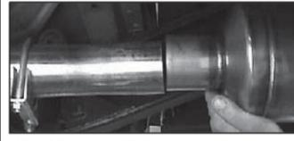
15. With the JBA logo to the rear of the vehicle, slip muffler (B) on head pipe (A). NOTE: You may have to tap it with a rubber mallet.
