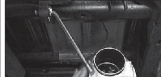
16. Slip rear muffler hanger (F) over rear slip joint of muffler (B) and hand tighten at this time.
