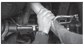
6. Remove tail pipe assembly from the rear of vehicle.
