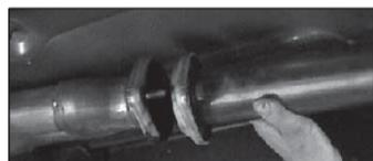
12. Install head pipe over studs and install flange nuts and align flange. using a 15mm socket and ratchet, tighten nuts completely. NOTE: we recommend using anti-seize on threads.
