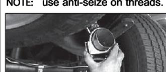
21. Install 3" clamp (G) over end of tail pipe (C).
