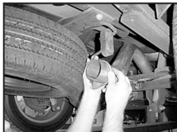
8. Slip tail pipe hanger clamp (E) over tail pipe (B) and insert hanger into factory rubber isolator.
