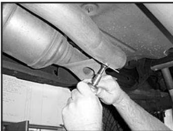
4. At the front of the muffler, cut through the welds and gusset. Remove muffler. Cut left side of gusset loose to allow for adjustment later.
