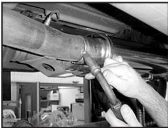
5. Install new muffler (A). Slip muffler onto converter pipes with minimum overlap. Tack weld in place.
