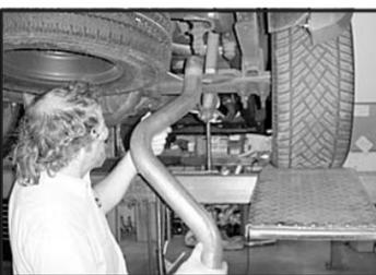
6. Install tail pipe (B) from the rear of vehicle.
