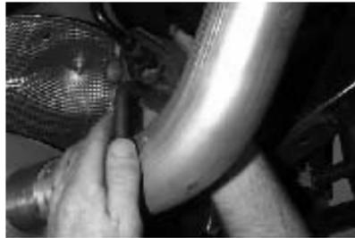
11. Insert the tail pipe hanger into the rubber grommet behind the muffler.
