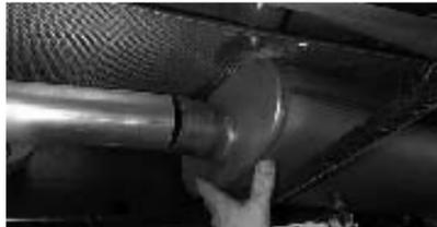
7. Install the new JBA muffler (B) onto the intermediate pipe (A) and then position the 3" clamp over slip connection.
