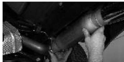
15. Align the tip and resonator and slide the 3" clamp with hanger over the slip connection.
