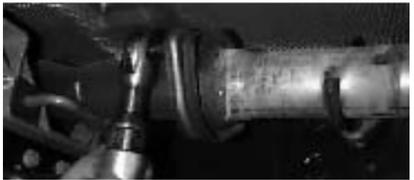
4. Remove the nuts attaching the intermediate pipe to the catalytic converter assembly using a 9/16" deep socket.
