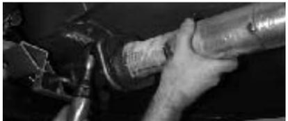
7. Using a 9/16" deep socket, attach the intermediate pipe to the catalytic converter assembly.
