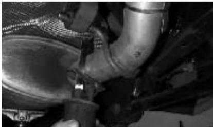
3. With vehicle raised and properly supported, using a reciprocating saw or hack saw, cut the tail pipe approximately 3" behind the muffler.
