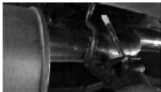
3. With vehicle raised and properly supported, using a reciprocating saw or hack saw, cut the tail pipe approximately 1" behind rear muffler hanger.
