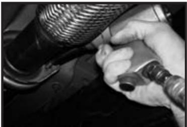
4. Remove nuts attaching muffler assembly, remove hanger rods from isolators, remove muffler assembly from vehicle
