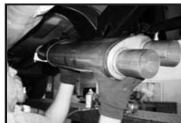
10. Install muffler onto intermediate pipe to insure full insertion. Align so tailpipes are flat
