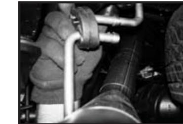
19. Install rubber isolator onto frame bracket. Install hanger rod into isolator adjust axle pipe & turnout together to clear bed crossmember, spare tire, leaf spring, etc. \*\*Some "adjusting" of brake line bracket will be necessary. "Adjust" to allow 2" of clearance between brake line and exhaust pipe as a minimum
