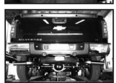
21. Adjust exhaust system to adequate on all components and achieve a symmetrical appearance. Tighten all fasteners & clamps securely
