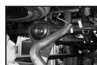
11. Install right-hand axle pipe. Insert into right-hand muffler outlet. Mark to ensure full insertion
