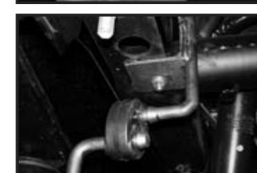
16. Install left-side rear frame bracket into existing hole in frame, behind tubular crossmember using hardware provided.
