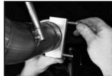
15. Install clamp on slip joint. Position to clear spare tire and leaf spring. Align tailpipe to clear shock, spare-tire, and bed crossmember. Snug clamps lightly.
