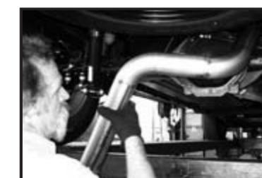
17. Install left-side axle pipe with hanger rod forward. Slip into muffler, mark to insure full insertion.
