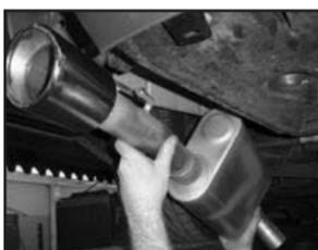
12. Install the muffler with tip assembly (D) onto the passenger side head-pipe (B).
