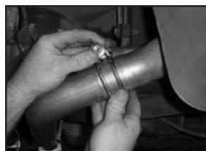
14. Align the new tips of the system for proper clearance from rear valance. Secure in place by tightening clamps (G) and (H).
