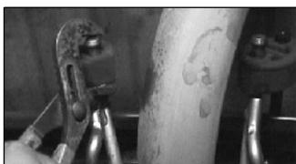
8. Spray lube on two rear muffler hanger rods, and remove from lower holes in rubber grommets using channel lock pliers.
