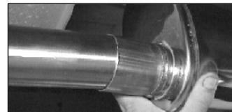
13. Install muffler (B) with offset end forward and down. Slip on 2".
