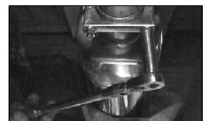
17. Install and position rear muffler 2 1/2" clamp (E) over slip joint and tighten completely using a 9/16" deep socket. NOTE: Use anti seize on threads of clamp. See Notes #2
