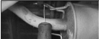
3. With vehicle raised and properly supported, support muffler and cut off tail pipe 4" behind rear of muffler. See Notes: #1
