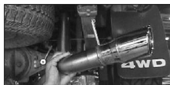
15. Install tail pipe (C) from rear of vehicle, and slip rear tail pipe hanger rod into lower hole in rubber grommet.
