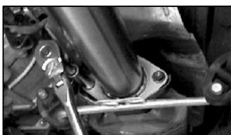
11. Bolt JBA head pipe (A) to flange using 14mm socket. NOTE: Oxygen sensor flange points inward.
