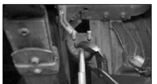
4. Spray lube on rear tail pipe hanger rod, and remove from rubber grommet using channel lock pliers.
