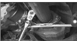
7. With muffler properly supported, remove two flange bolts in front of muffler assembly using a 14mm socket. Save bolt's they will be reused.
