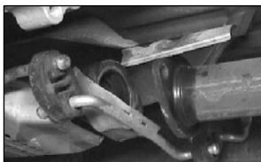
9. Remove muffler assembly, taking care not to damage flange gasket.
