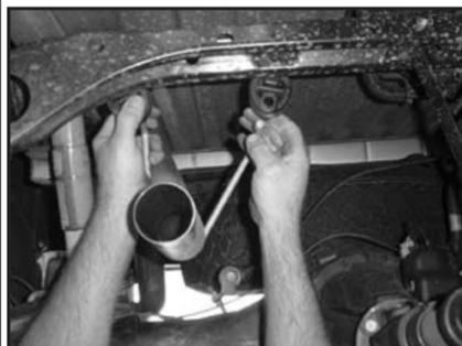
10. Insert front tail pipe hangers into factory rubber isolators.
