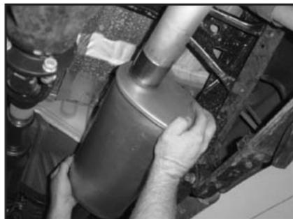
11. Slip muffler (B) into the tail pipe (C) as shown in the photo.
