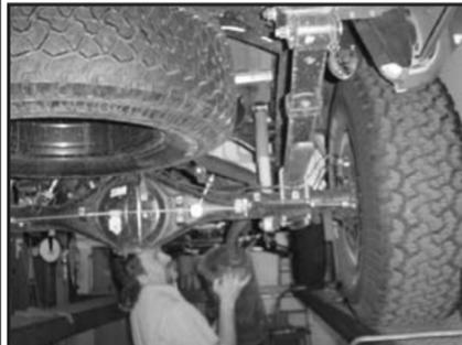
8. Remove factory exhaust from the vehicle.
