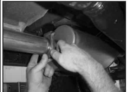
15. Insert intermediate pipe (A) into muffler (B) and install exhaust clamp (D) at the front of the muffler (B).
