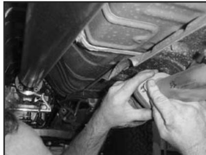
13. Install and secure the new intermediate pipe (A) into the vehicle by reinstalling the factory Catalytic Converter bolts and nuts.
