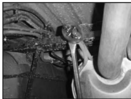
5. Using the pry bar, remove the tail pipe hangers from the rubber isolators.
