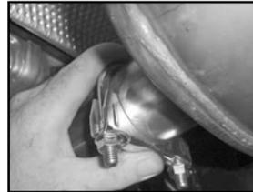
12. Slip the rear offset end of the JBA muffler (B) into the muffler clamp with hangers (F). The offset end of the muffler should be toward the center of the vehicle.
