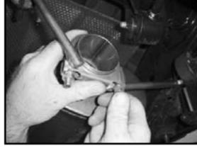
13. Slip the turn up pipe (C) onto the JBA muffler (B). Position muffler clamp with hangers (F) over connection and tighten.
