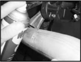
4. Unbolt the factory tail pipe above the rear axle.
