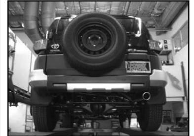
17. Using a soft cloth, remove all prints from exhaust tip.
