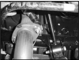
5. Using channel lock pliers remove the tailpipe hanger from the rear rubber isolator and remove the tailpipe from the rear.
