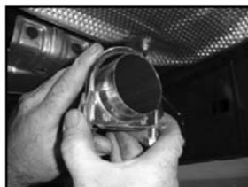
10. Install the muffler clamp with hangers (F) into the rear (2) muffler hanger rubber isolators with the hangers shifting pipe to driver side.
