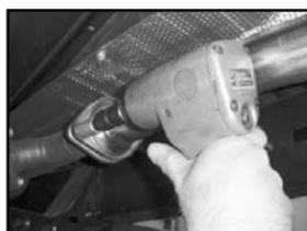
9. Slide one of the supplied 2-1/2" exhaust clamps (E) over the end of the JBA intermediate pipe (A).
