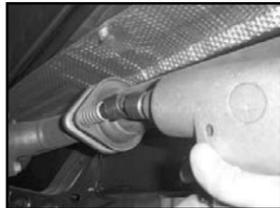
7. Using channel lock pliers remove the rear muffler hangers from the (2) rubber isolators and remove the intermediate pipe / muffler assembly from the vehicle.
